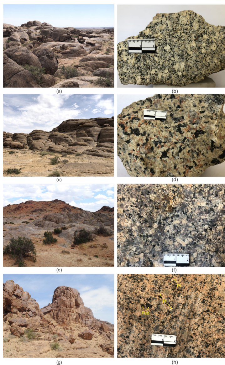
Figure 3: Outcrop and hand specimen photos of alkali granites in the Western body of Khanbogd pluton. Note: (a) outcrop of intrusion I-W; (b) coarse-grained porphyritic texture greyish color aegirine-arfvedsonite granite in intrusions I-W; (c) outcrop of II-W, where dominated horizontal platy joint; (d) elpidite rich agpaitic, greyish color granite in intrusion II-W; (e) outcrop of III-W, intruded into II-W; (f) reddish color aegirine-arfvedsonite granite in III-W; (g) outcrop of IV-W, where cubic shape is formed from set of vertical and horizontal joints; (h) red color, ferro-edinite granite.
